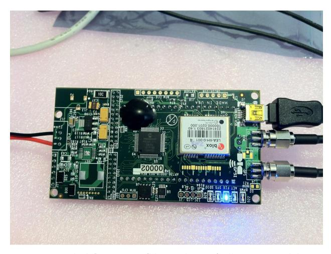
4. Start uCenter, select the "Receiver->Port->XXX" where XXX is the USB port found by your computer attached to GPS1. NOTE: you can use DeviceManager under Windows and find the uBlox USB Device port.
