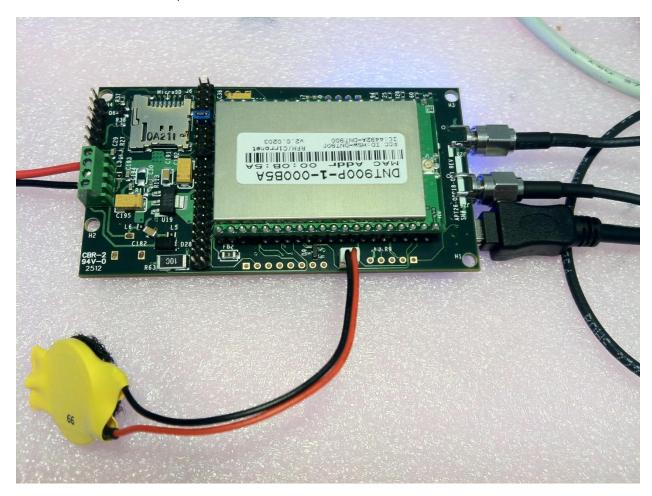
3. Connect a mini-USB cable to the GPS1 USB port and the other side to the computer
