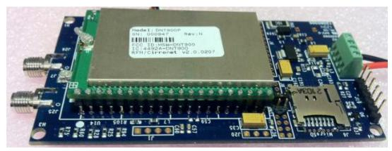
The GPS-1 telemetry module is a high performance, secure, tracking, monitoring, and data logging system which enables tranmission of GPS position and telemetry data up to 100 miles LOS (Line of sight) to the Base-station-1 or Base-station-2 receiver. It also features local logging of all sensor and GPS data onboard Micro-SD storage..
